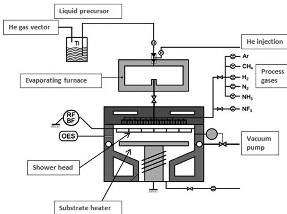
Figure 1. Schematic representation of the 300 mm AltaCVD 300 chamber.
