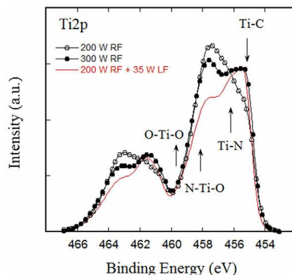
Figure 13. XPS Ti2p spectra of TiN samples.
