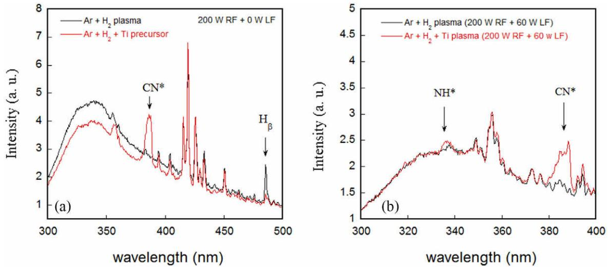
**Figure 7.** (a) A comparison for a 200 W RF plasma with and without a Ti precursor. (b) The impact of the Ti precursor for a 200 W RF + 60 W LF plasma.
