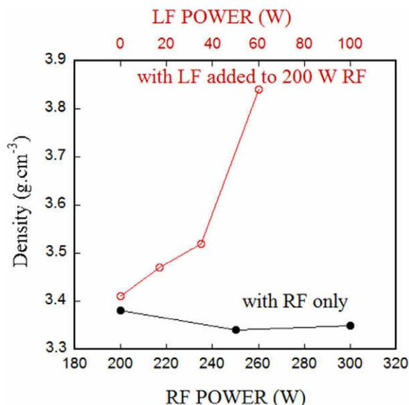
Figure 12. TiN density in RF mode and DF mode with LF addition.
