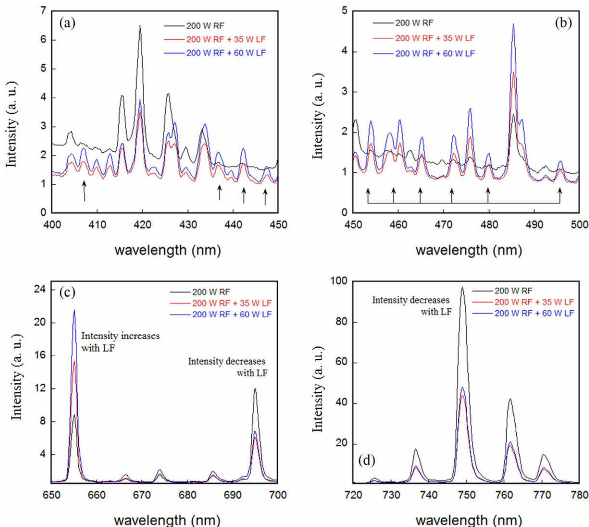
**Figure 5.** The impact of LF addition in Ar + H<sub>2</sub>OES in four spectral ranges: (a) 400–450 nm; (b) 450–500 nm; (c) 650–700 nm; and (d) 720–780 nm. Arrows in the figures indicate new emission peaks.
