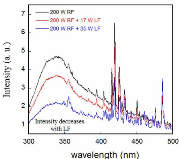
**Figure 6.** The impact of LF addition in Ar + H<sub>2</sub>OES in the 300–500 nm range.
