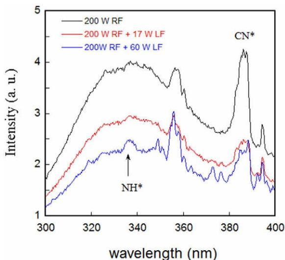
**Figure 9.** Evolution of the OES of Ar + H<sub>2</sub>+Ti precursor plasma with LF power.
