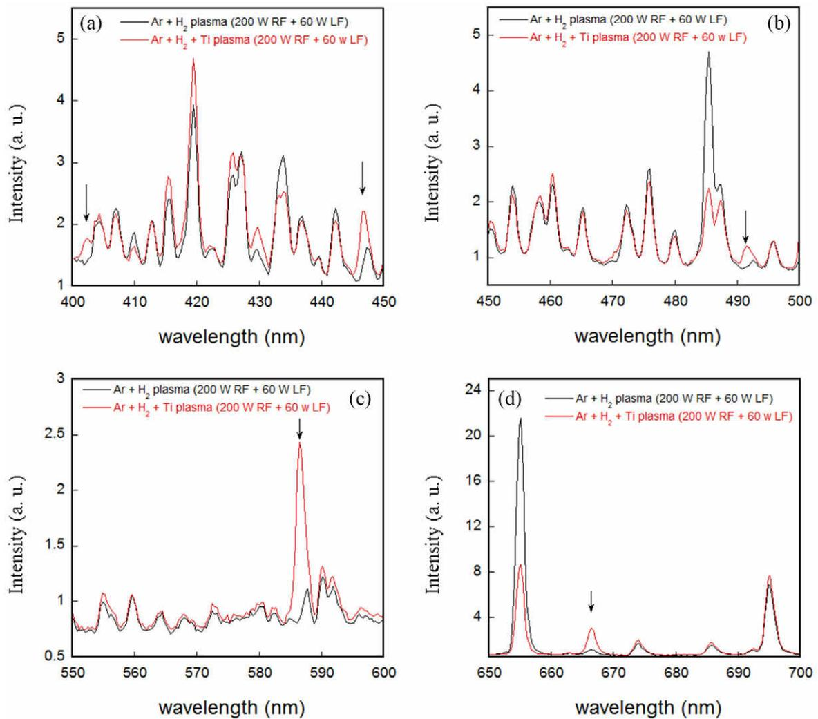
**Figure 8.** Effect of Ti precursor addition in the OES of the 200 W RF + 60 W LF plasma: (a) the 400–450 nm range; (b) the 450–500 nm range; (c) the 550–600 nm range; (d) the 650–700 nm range.
